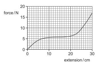
What is the best estimate of the strain energy stored in the rubber band when it is extended  $30 \, \text{cm}$ ?
