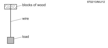
By how much would a wire of the same material, but of diameter 2*D* and length 3*L*, extend when the same load is applied?
