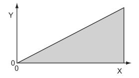
The shaded area represents the total strain energy stored in stretching the wire.
