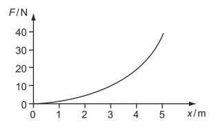
The energy stored in the rubber for an extension of 5 m is
