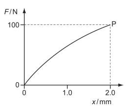
What could be the value of the strain energy stored in the wire when it is stretched to point P?
