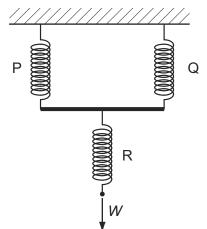
Springs P and Q are identical and have spring constant k. Spring R has spring constant 3k.
