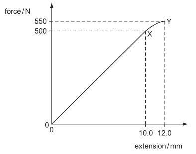
What is the total work done in stretching the sample from zero extension to 12.0 mm? Simplify the calculation by treating the region XY as a straight line.
