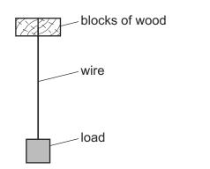
By how much would a wire of the same material, but of diameter 2D and length 3L, extend when the same load is applied?
