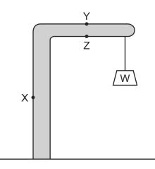
A weight W is lifted by a rope at the end of the beam.
