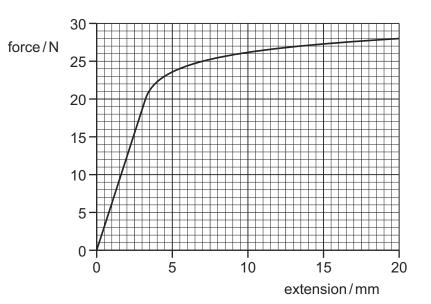
How much work needs to be done by the tensile force, to two significant figures, to cause an extension of 7.0 mm?
